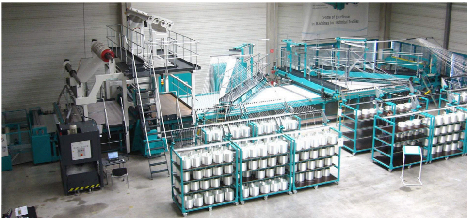
Figure. 2.5: Warp knitting machine for manufacturing of non-crimp fabrics [68]
