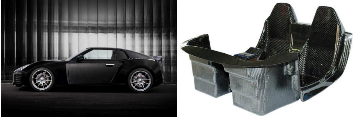
Figure. 1.2: Roding roadster and its RTM chassis
