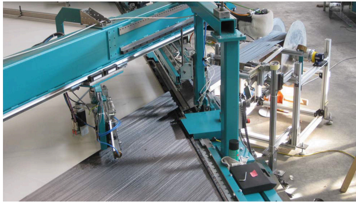
Figure. 2.6: Fiber spreading and placement during NCF manufacturing [68]
