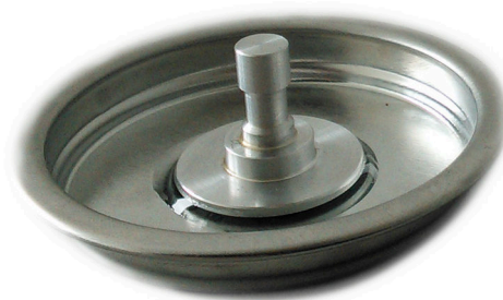
Figure. 5.14: Specimen holder for viscosity measurement
