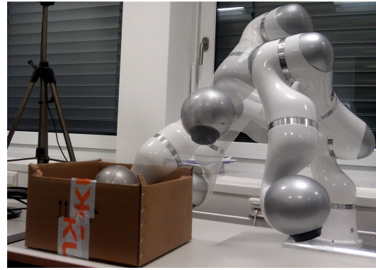
Fig. 1. The KUKA Light-Weight-Robot IV+ goes in and out of a box avoiding collisions. This task is useful, for example, to ask the robot to take something in the box.
