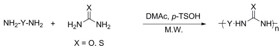
Scheme 1.6. Schematic representation for the general synthesis of polyureas /polythioureas organocatalyzed by p -TSOH.
