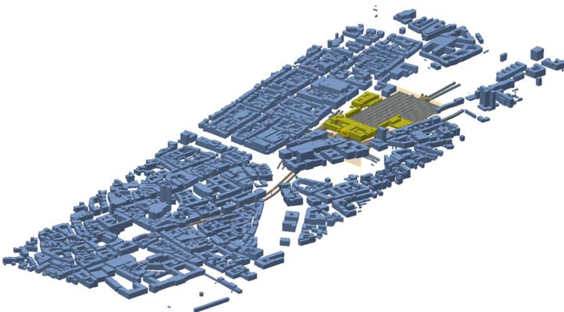
Figure 22: Integration of the multi-scale shield tunnel model with the 3D city model of Munich
