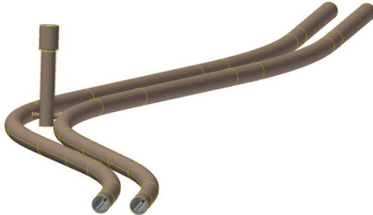
Figure 21: A model of an escape shaft between the two tunnel tubes
