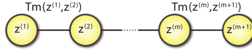
Figure 2.5: Concept of a Markov chain with regard to the random variables \mathbf{z} . Each random variable \mathbf{z}^{(m+1)} exclusively depends on its predecessor \mathbf{z}^{(m)} with the transition probability Tm(\mathbf{z}^{(m)}, \mathbf{z}^{(m+1)}) .
