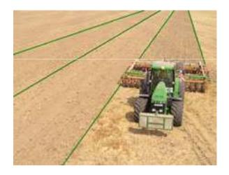
Automatically steers the tractor via hydraulic valve and becomes part of the machine.
