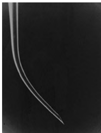
(a) Curved glass micropipette with beveled tip [8]
