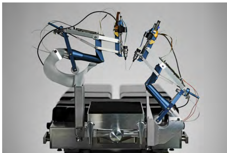
Figure 2.3: RCM mechanism designed and developed at Technical University of Eindhoven, Netherlands
