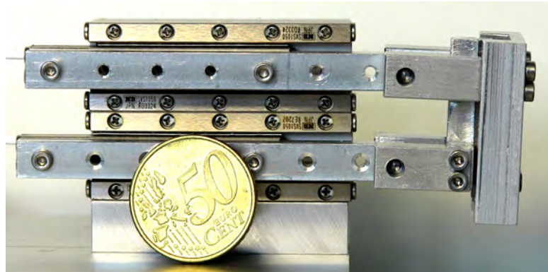
Figure 4.2: Parallel Coupled Joint Mechanism (PCJM), developed as the main joint mechanism of the robot for ophthalmic surgery [84].
