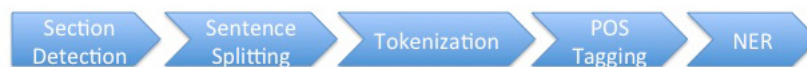
Figure 5.1: Simplified version of an information extraction pipeline that can be used for relation extraction in single-slot tasks.
