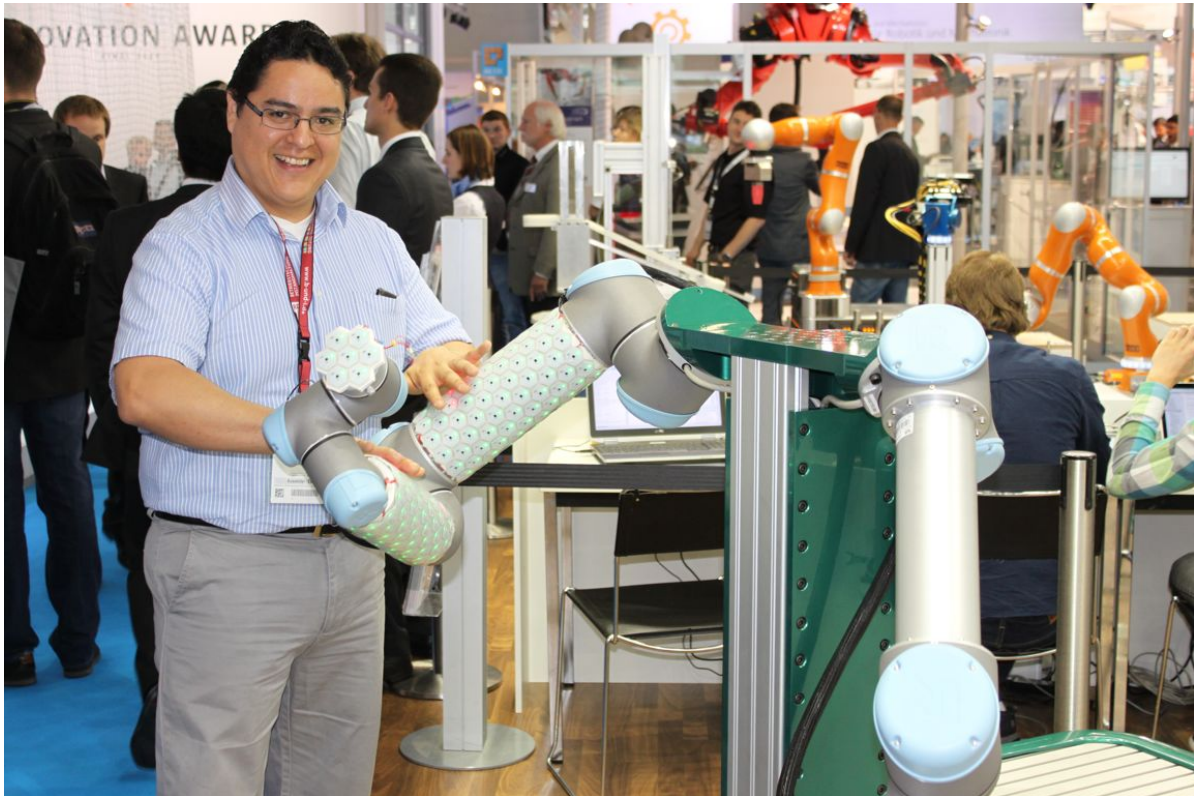
FIGURE 6.29. The figure shows the robot TOM on the trade fair Automatica 2014, visually displaying the contact states detected on its surface.
