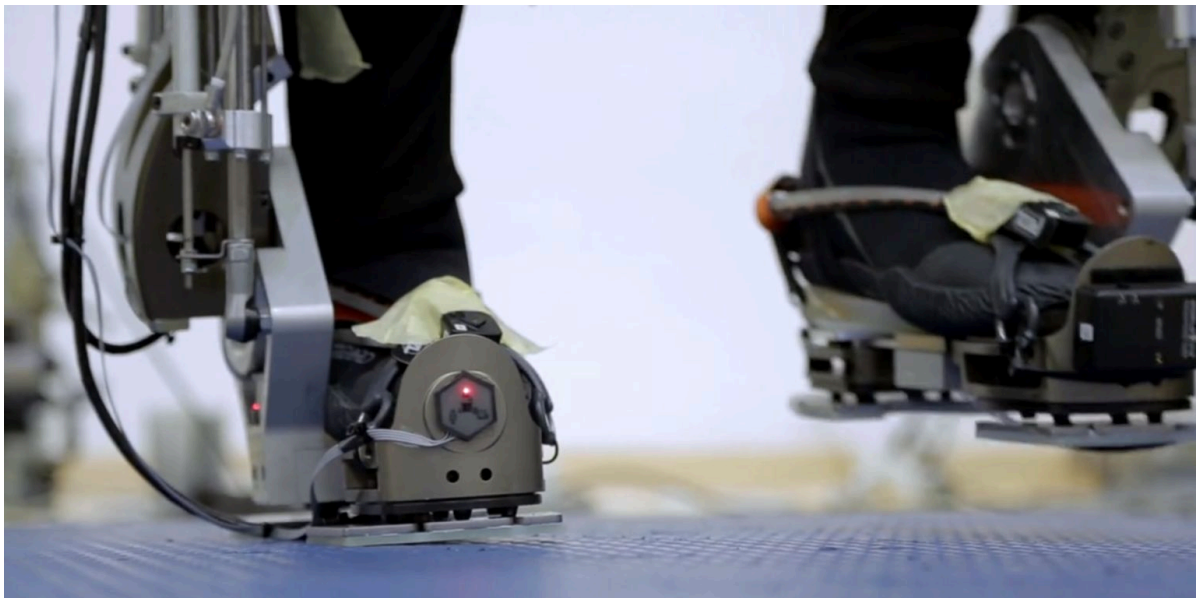
FIGURE 6.17. The figure shows a skin cell of CellularSkin™ mounted on the tip of the exoskeleton shoe for contact detection with the soccer ball.
