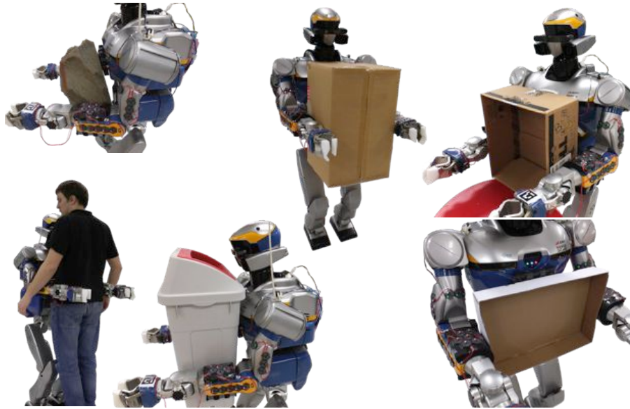
FIGURE 6.2. The figure shows HRP-2 holding objects that have been grasped only with tactile feedback and a self-explored body model. Key poses for the trajectory generation and expected contact points have been taught with a novel method of tactile human-robot interaction.
