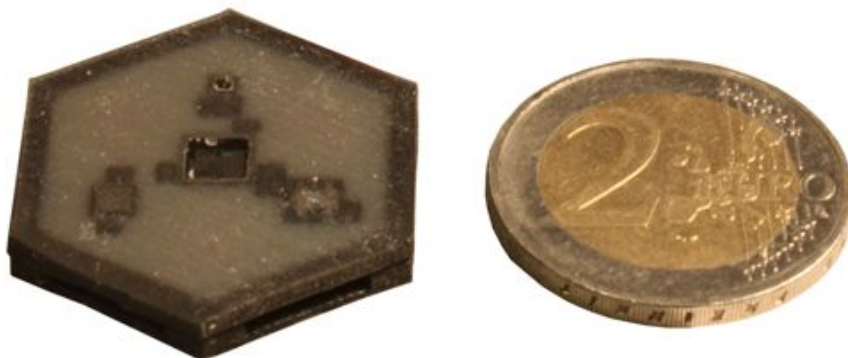
FIGURE 3.10. The figure shows the size of skin cell version 2.0 compared to a 2 EUR coin.
