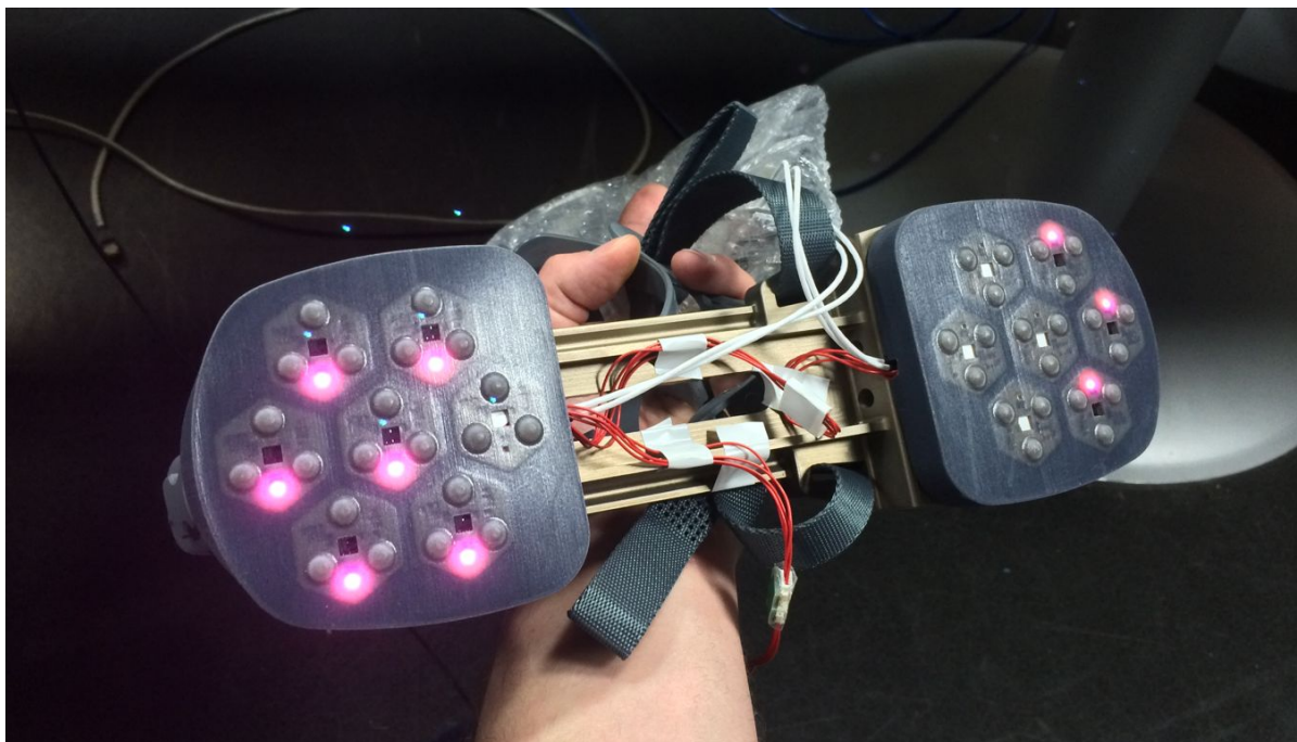
FIGURE 6.15. The figure shows the shoe sole of the exoskeleton, equipped with CelluARSkin™.
