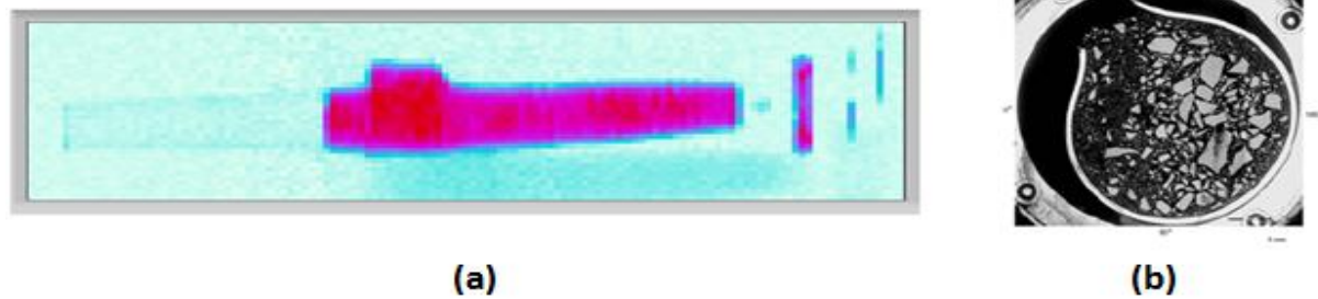
Figure 1.3: IFA-650.4 fuel rod status after the test a) Neutron Radiography [16]; b) Destructive test fuel cross section analysis [16]
