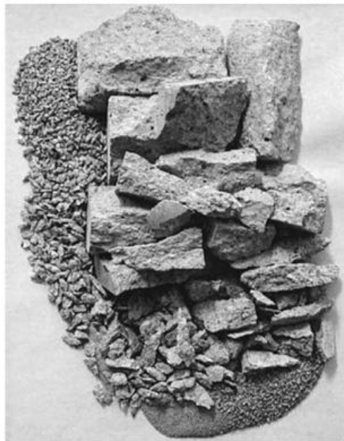
Figure 4.2: Concrete fragments derived from crushing Figure from Reference [3]
