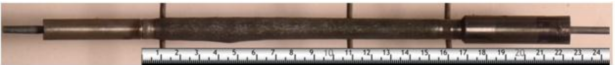
Figure 3.22: Visual inspection Rod 2 (90 orientation)
