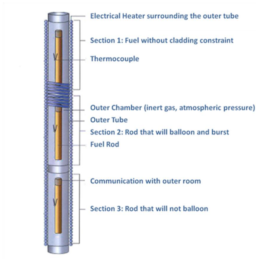
Figure 2.10: Preliminary design based on the conceptual separate effect test
