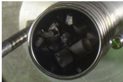
Figure 4.1: Rod 2 fuel fragments during sifting operation
