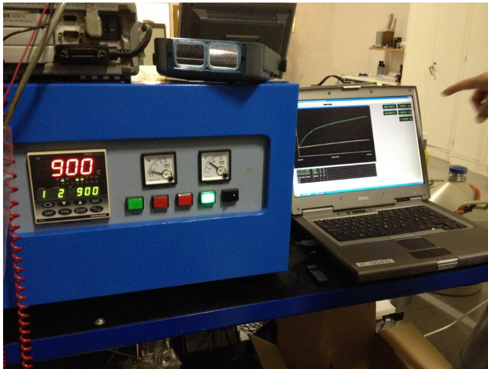
Figure 3.15: Data acquisition system during the experiment Electric oven at the target temperature of 900°C
