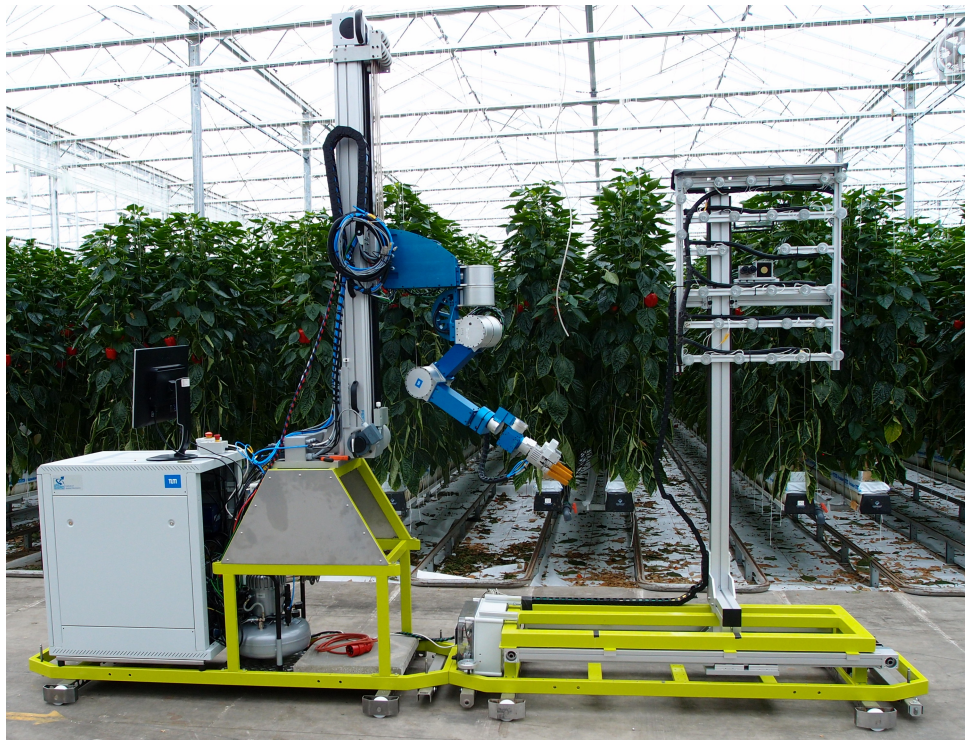
(a) Integrated system for sweet pepper harvesting.
