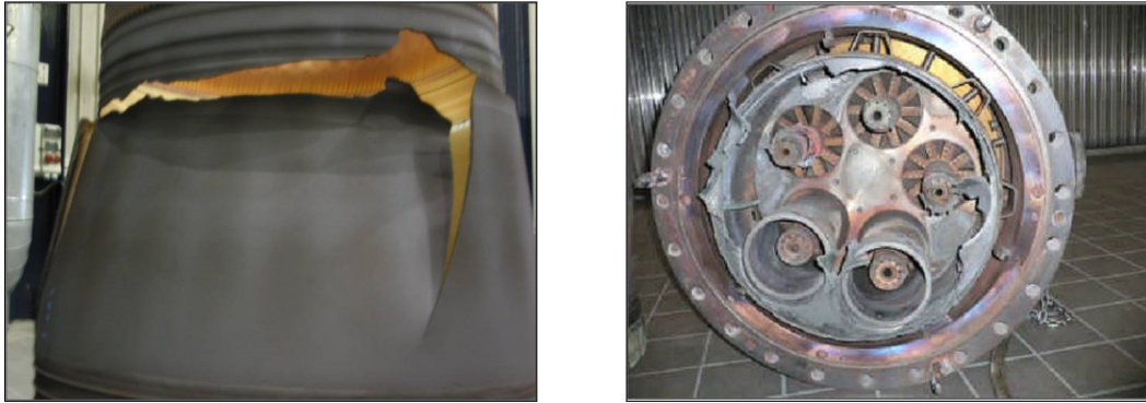
Figure 1.1: Gas turbine parts – a connecting piece (left) and a burner assembly (right) – damaged by combustion induced oscillations; courtesy of Laborelec/GDF–Suez.
