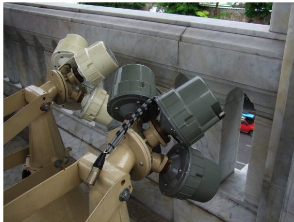
Figure 6.5: Multiple drivers connected to a single horn increase the volume that can be modulated by loudspeaker actuation.
