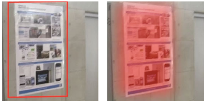
Figure 5.3: Highlighting of interaction points for context-based services. Instead of framing objects (left), we propose a soft border visualization (right) for less sensitivity to jitter and to reduce distraction of the user.
