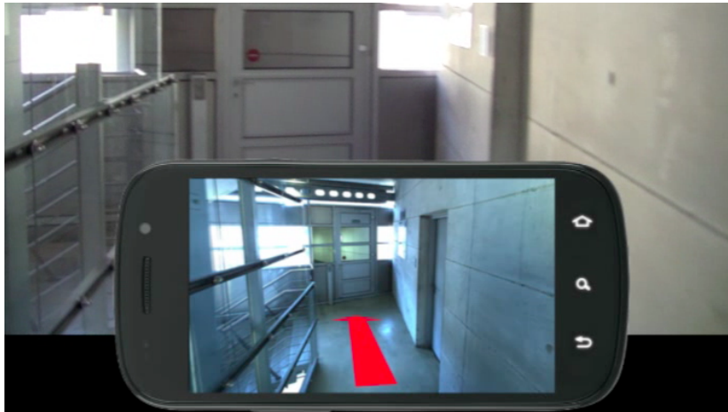
Figure 5.4: A screenshot from one of the videos used in the study, showing a mockup of the indoor navigation system. The upper part shows the simulated field of view, the smartphone screen the simulated navigation system output.
