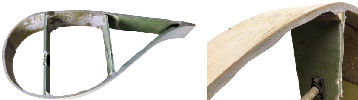
Fig. 5.2: Wavy spar cap laminate [56]
