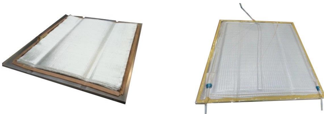
Fig. 5.23: Fabrication method: draped preform (left); ready for infusion (right)
