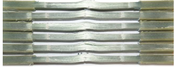
Fig. 5.34: Failure mechanisms - delamination and fiber failure of a tensile loaded specimen
