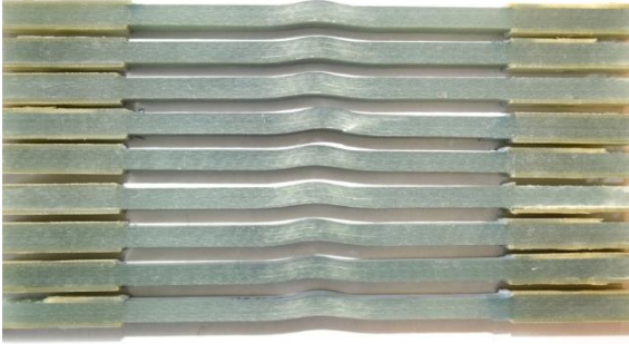
Fig. 5.34: Failure mechanisms - delamination and fiber failure of a tensile loaded specimen
