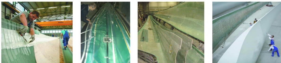
Fig. 2.20: Process steps: Draping, infusion and curing, assembling and finishing [32]
