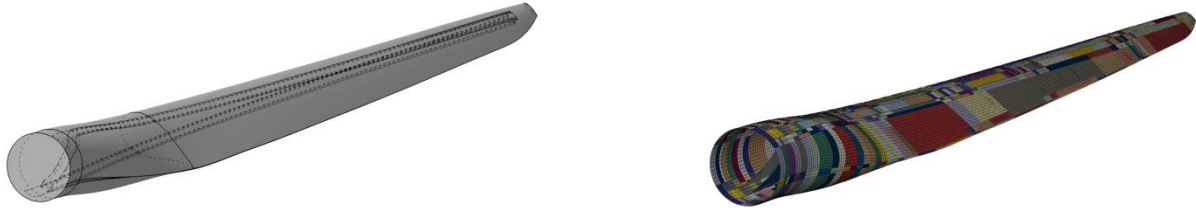
Fig. 3.14: CAD-model (left); FE-model (right)
