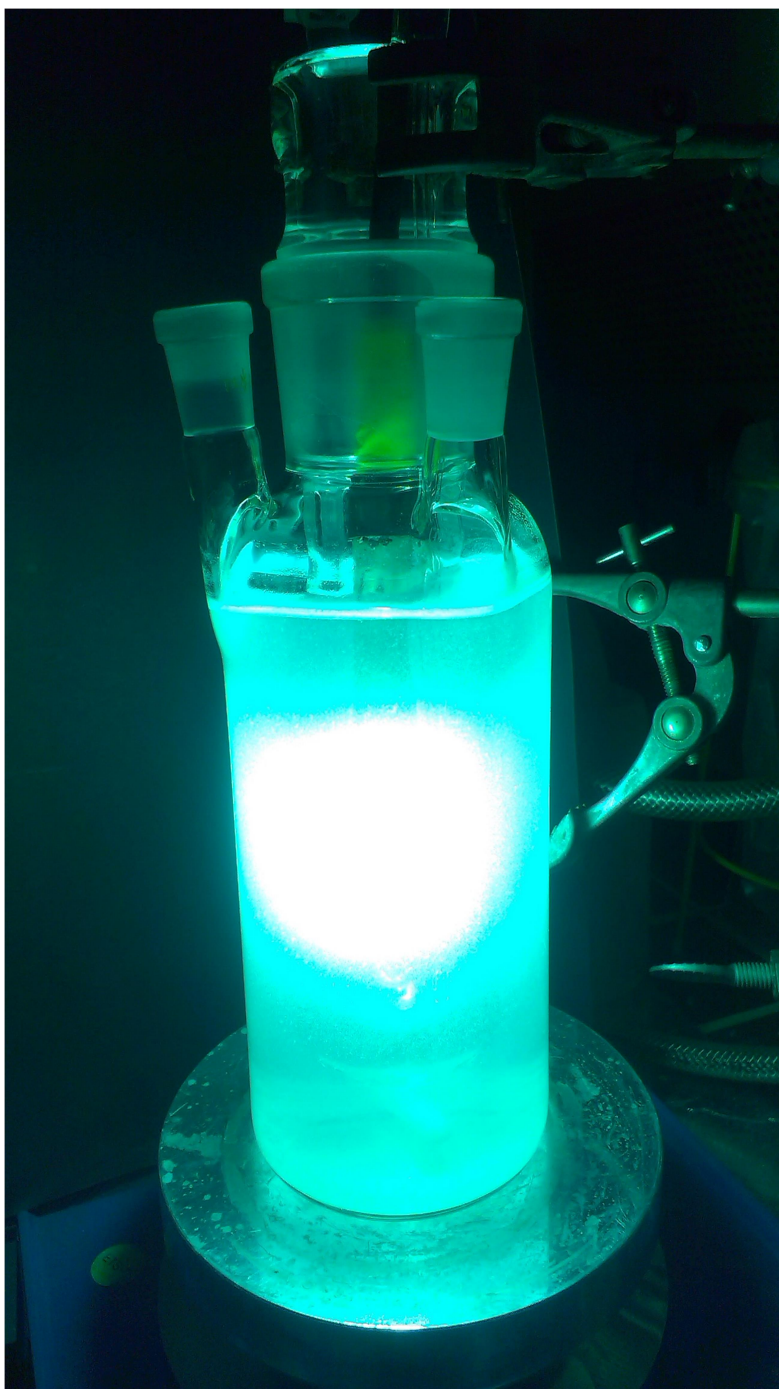
Figure 25 An illustration of the cylindrical glass tube reactor on a magnetic stirrer. The two inlets were sealed during irradiation.
