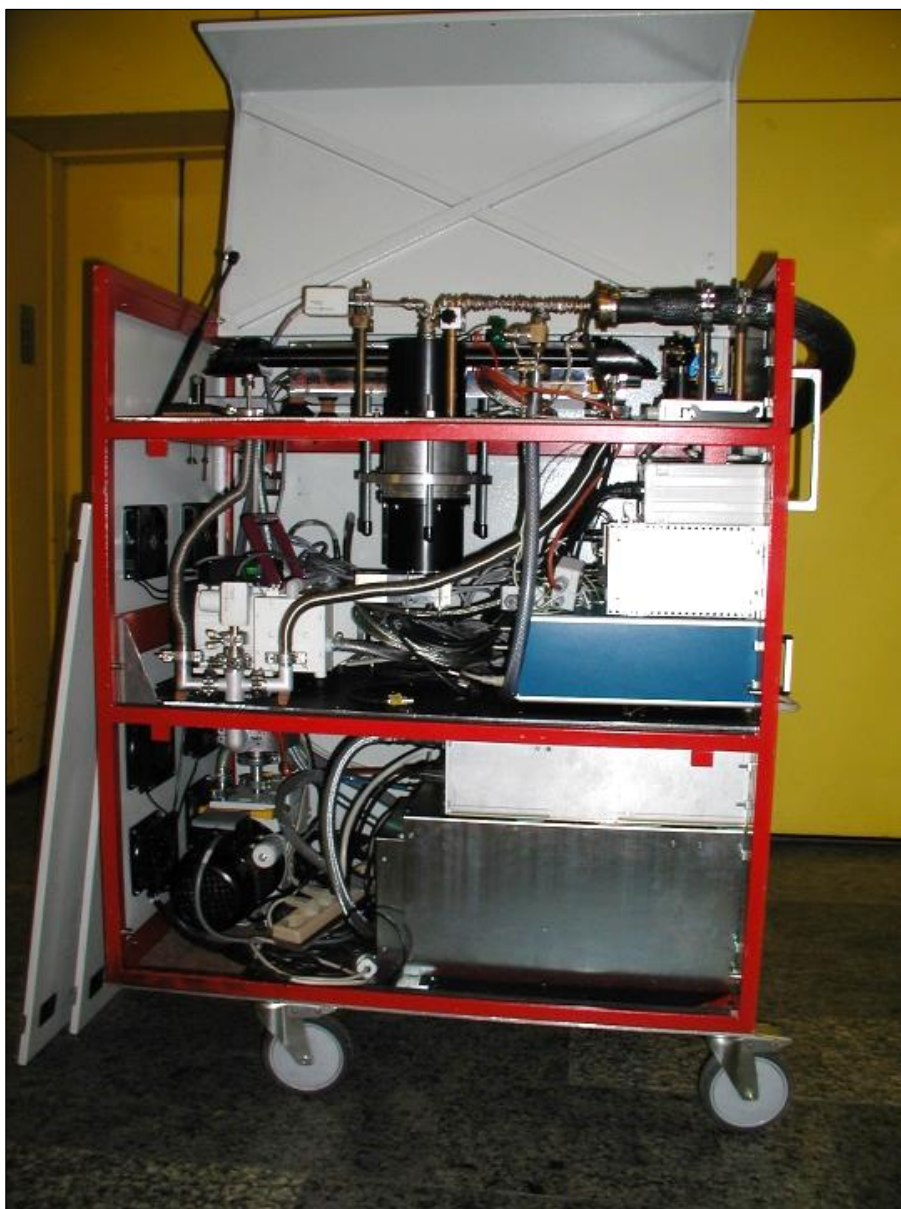
Figure 6.4. Picture of the prototype-III destined for use at BMW-AG. Upper floor contains: OPO laser, FC, power meter, spectrometer, optical path, gas inlet system with the GDC and the heated stainless steel pipe. Medium floor contains: the optical collection system, filter, PMT, membrane pump, two power supplies (GDC and PMT), two heating controllers, pressure reader and flow meter. Lower floor contains: laser power supply, laser cooling unit, penning, rotatory pump with zeolite filter and several multi-sockets.
