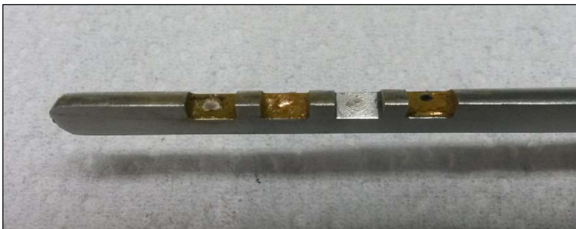
Figure 14.10. Detail of the sampling tip after desorption.
