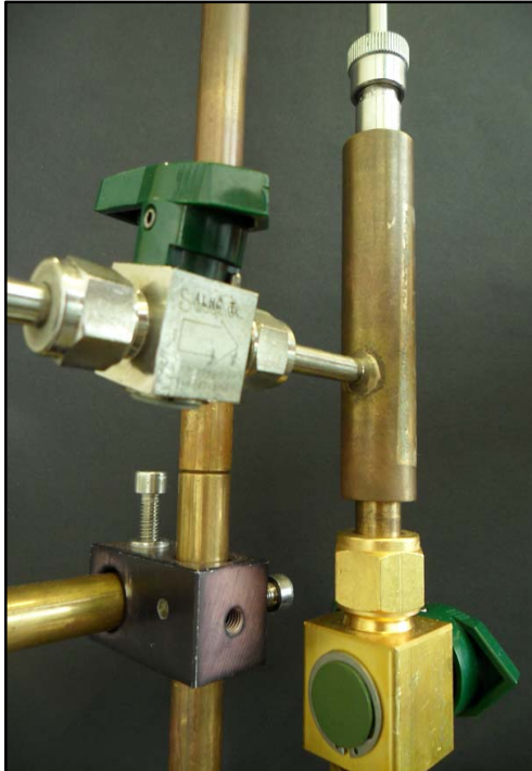
Figure 13.7. Manipulator. The sampling rod is sealed with an Ultra-Torr fitting.
