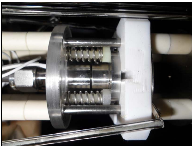
Figure 13.4. Detail of the Parker® valve and the Teflon® block.
