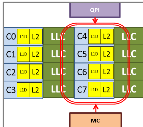
Figure 3.13: Sandy Bridge-EP Architecture. LLC stands for last level cache, also known as L3 cache.
