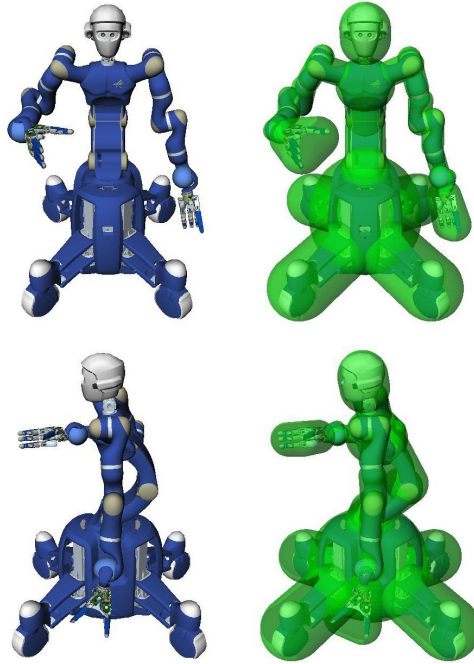
Figure 3.2.: Geometric collision model of Rollin' Justin consisting of 28 bounding volumes (left arm: 8, right arm: 8, mobile base: 5, torso: 4, head: 2, floor: 1). The volumes are spheres, rounded cylinders, and bodies obtained by unrolling spheres on triangles.
