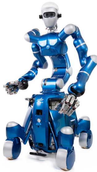
Figure 1.1.: Wheeled humanoid lightweight robot Rollin' Justin developed at the Institute of Robotics and Mechatronics at the German Aerospace Center (DLR)
