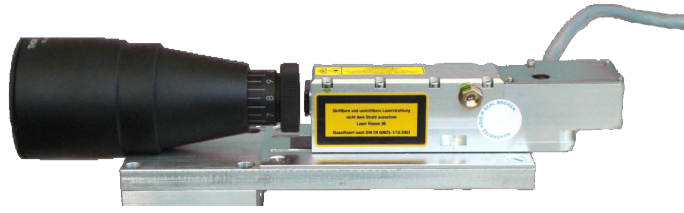
Figure 5.5: LIDAR laser with 10x beam expander. The laser is a frequency doubled Nd:YAG with 1\mu\text{J} pulse energy and 500 ps pulse duration and can be fired at rates up to \sim 2\text{kHz} . The 10x beam expander helps to reduce the light flux density, in order to enhance eye safety and to reduce the beam divergence to about 0.05^\circ .
