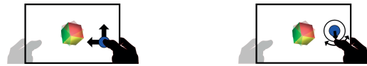
Figure 1: One thumb rotation of the virtual trackball approach (left) and the 2D rotation (right).
