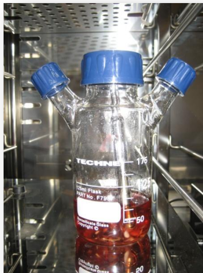
Image 6: Spinner Flask for Chondrocyte Isolation
