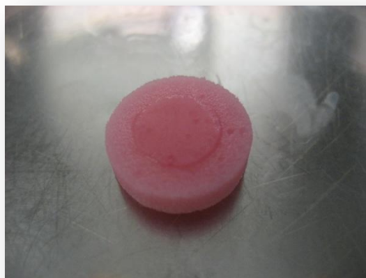
Image 13: Cell-Seeded PU Scaffold with PU Ring
