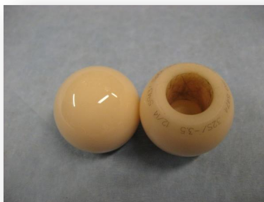
Image 10: Ceramic Hip-Ball used for in vivo simulating Loading
