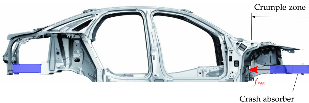
Figure 7.1: Crash absorbers shown within the crumple zone of the AUDI SPACE FRAME
