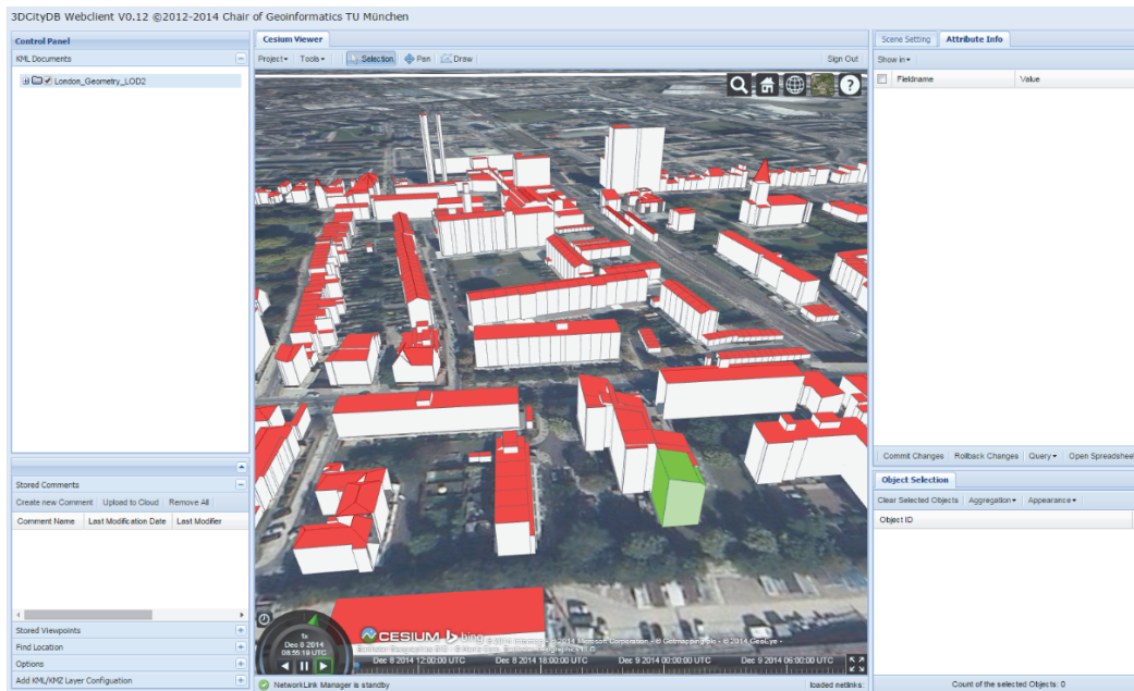
Figure 10: 3D web client displaying extra structure information of LOD2 building of London dataset
