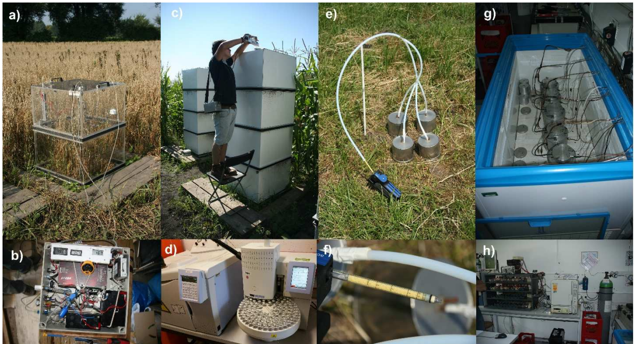
Figure 8 Different Measurement systems and analyzing units for the determination of soil gas fluxes which were used in the present study. a) Closed dynamic manual chamber system for the determination of NEE (transparent chamber) or R_{eco} (opaque chamber, not shown) coupled to an b) infrared gas analyzer (IRGA, LI-820); c) Closed static manual chamber system for the determination of N_2O and CH_4 fluxes. Gas samples were analyzed via a GC d) equipped with an FID and an ECD; e) Open dynamic chamber method (“Dräger-Tube Method” for the determination of NH_3 volatilization, NH_3 concentrations were analyzed via ammonia indicator tubes f); g) Helium-oxygen flow-through the chamber incubation system at the laboratory of the Institute of Landscape Matter Dynamics, Leibniz Centre for Agricultural Landscape Research (ZALF; Müncheberg, Germany) for the simultaneous determination of N_2 , N_2O , CO_2 and CH_4 fluxes in a controlled environment, h) concentration of N_2 were analyzed by a micro-GC equipped with a TCD. Concentrations of trace gases were analyzed by a GC equipped with an FID and an ECD.
