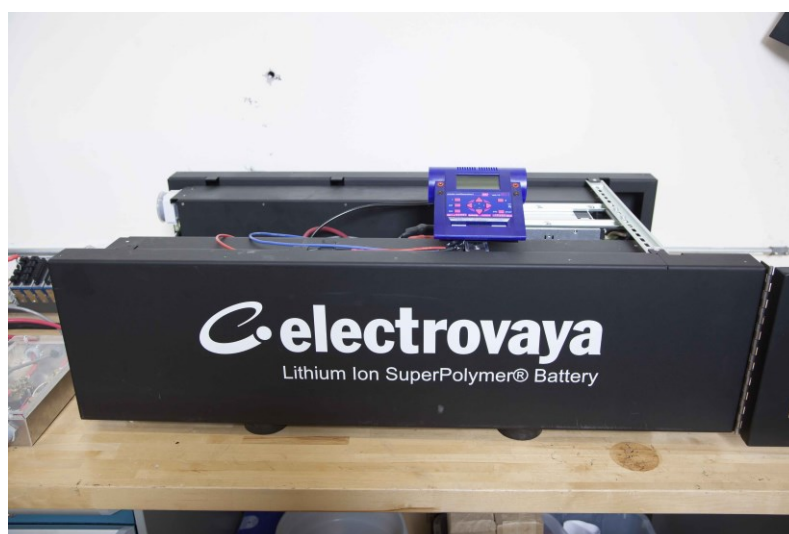
Figure 2-11: Residential storage battery built by the Canadian manufacturer Electrovaya
