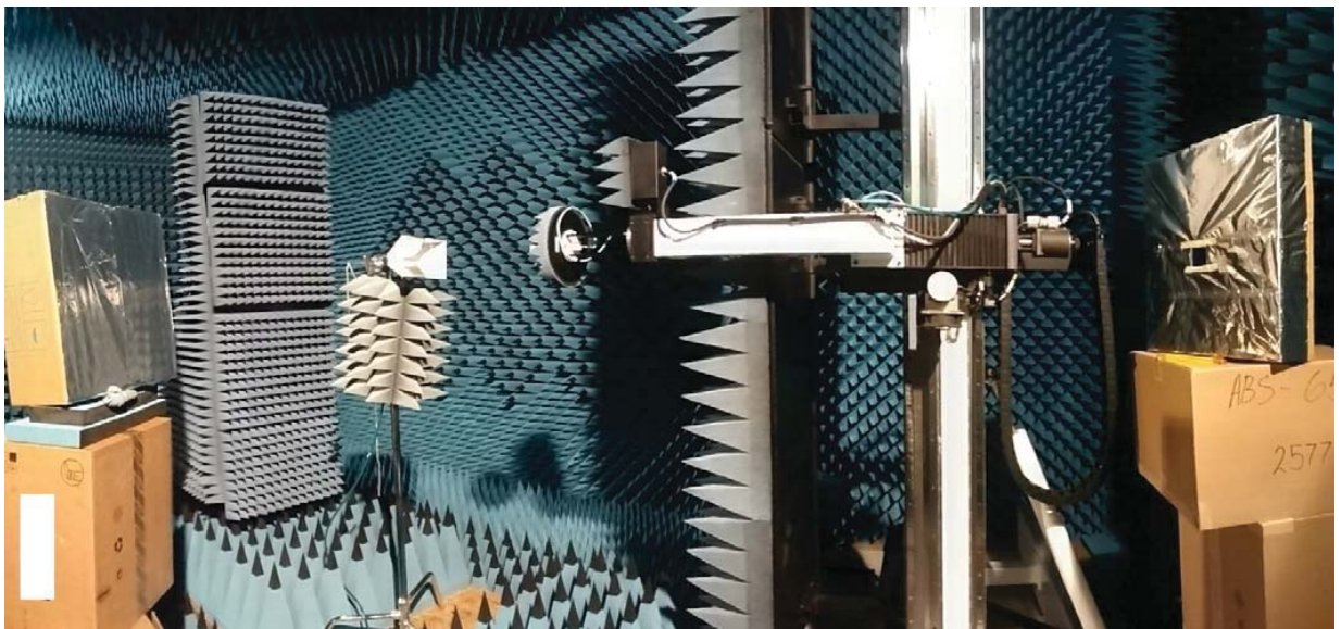
Figure 4.9: Two metal plates were introduced to the chamber in order to generate multipath contamination into the measurement data.
