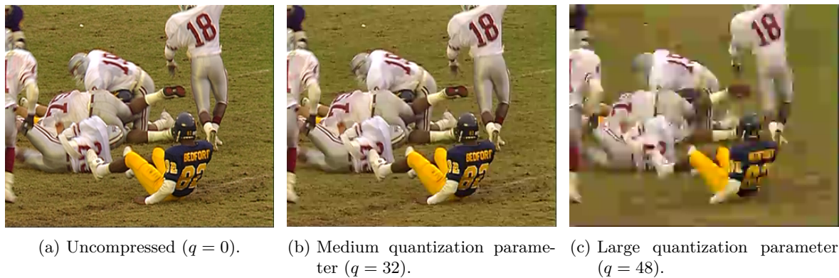
Figure 2.2.: Example frame of the Football video [Seq] encoded with H.264/MPEG-4 AVC using x264 [Vid] at different quantization parameter settings.
