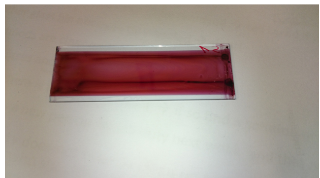
Figure 2: Polymer:fullerene film printed on glass substrate
