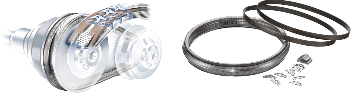
Figure 1.1: Pushbelt CVT ©BTT. It shows the two pulleys – each with a loose and a fixed sheave – and the pushbelt consisting of two rings and about 400 steel elements.
