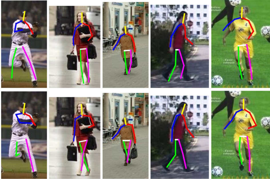
Figure A.6: Additional results on model refinement - PARSE : Additional results for the coarse-to-fine model using the cascade of ConvNets are presented from the PARSE dataset [187]. On the top row the result of a single ConvNet is presented, while on the bottom row the refined result using the cascade of ConvNets.
