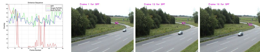
Figure 7.3: Failure of the Standard Particle Filter: (a): The overlap over time plot, based on the PASCAL VOC challenge [56] criterion, shows the performance of the SPF and the two versions of our method. Other images: SPF tracker gradually drifts due to collecting background information.
