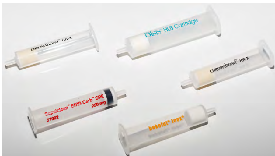
Fig. 13: Different types of disposable cartridges for solid-phase extraction (SPE) (Picture: Johannes Deyerling)
