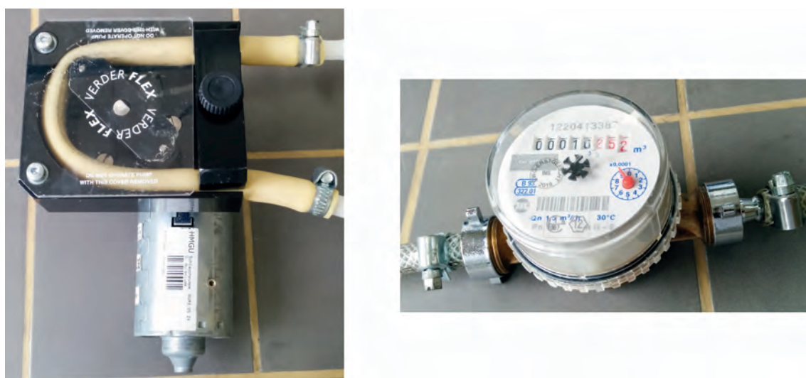
Fig. 22: OEM peristaltic pump (left) which is operated between 1 and 24 V DC either with battery or dedicated power supply and analog water meter (right)
