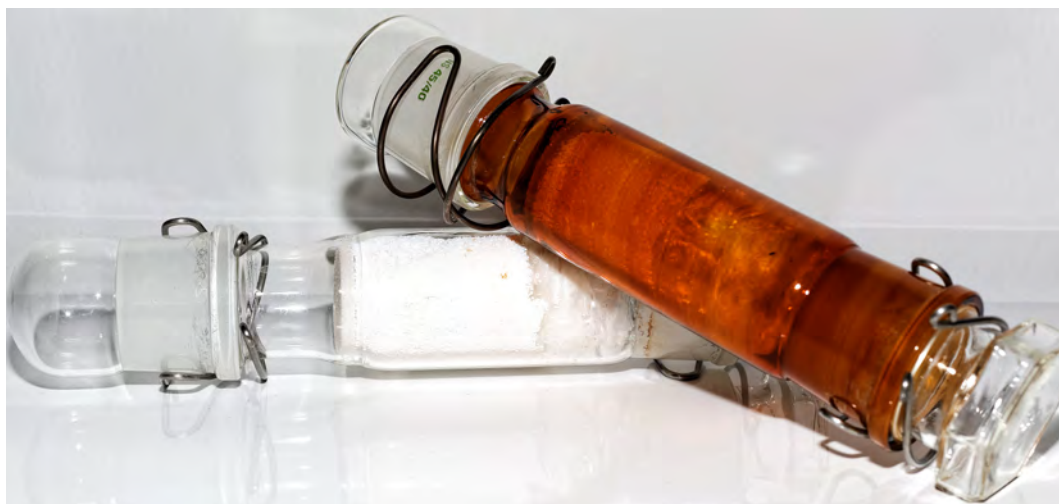
Fig. 21: Self-packed glass cartridge with XAD-resin trapped inside with glass frit and heat-treated glass wool (Picture: Johannes Deyerling)
