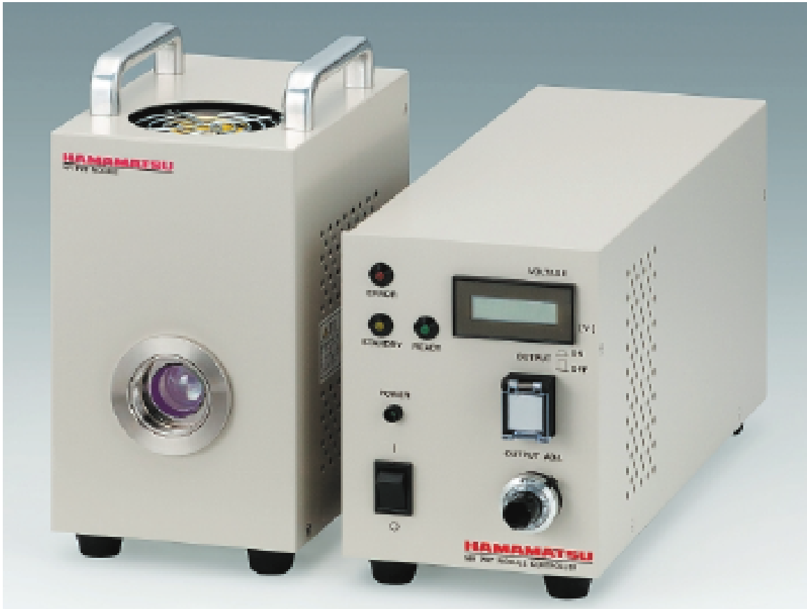
Figure 2.16: A photograph of the near-infrared photomultiplier (NIR-PMT, left) and the controller unit (right). On top of the NIR-PMT a ventilator can be seen which dissipates the heat produced by the Peltier elements which cool the photocathode. On the front side the BK7 (anti-reflective coated) condenser lens can be seen which focuses incoming parallel light onto the photocathode. The controller unit regulates the temperature of the Peltier elements, the power supply, and the high voltage of the NIR-PMT.
