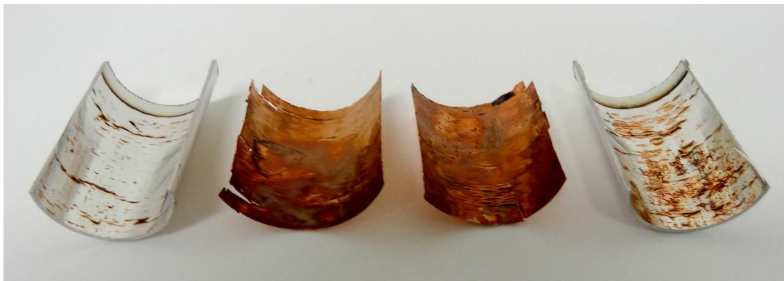
Figure 79: Copper deposited in two stages. Using a combination of low and high energy mode resulted in a removable copper foil. However, the foil was brittle and some copper remained on the substrate.
