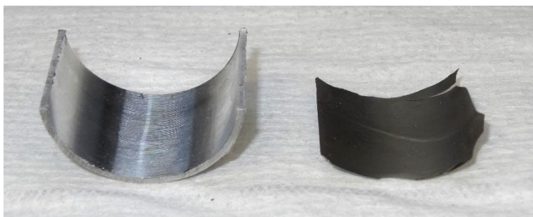
Figure 82: Al-U multilayer system. When using an aluminum interlayer between the substrate and the uranium layer, a bonding of the foil to the substrate can be prevented.
