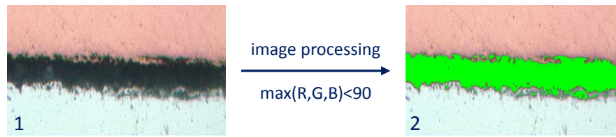
Figure 90: Image processing. The image processing algorithm detects gaps between the layers by analyzing the RGB color code of each pixel. Image 1 one shows a typical microscopic picture of a deformed target cylinder. In image 2, the gap found by the algorithm is marked in green.
