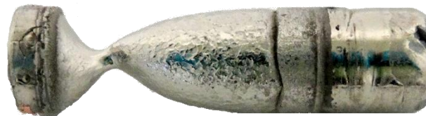
Figure 68: Nickel target burn-up. The burn-up profile of a cast nickel target shows a strong erosion on the upper half and almost no erosion in the lower part. The indentation in the lower part is a defect, which occurred due to a too rapid cooling during the casting process.
