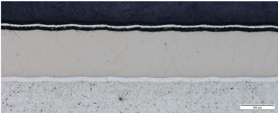
Figure 76: Al-U-Al multilayer system. The presented uranium layer was produced using a substrate temperature of 90°C and a sputter power of 90 W.
