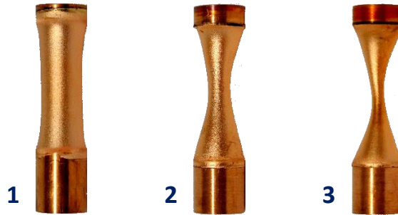
Figure 59: Copper target burn-up. Three different copper targets with different burn-ups are shown: 1) 0.6 \text{ cm}^3 \approx 5.4 \text{ g} , 2) 1.2 \text{ cm}^3 \approx 10.7 \text{ g} and 3) 1.5 \text{ cm}^3 \approx 13.4 \text{ g} .
