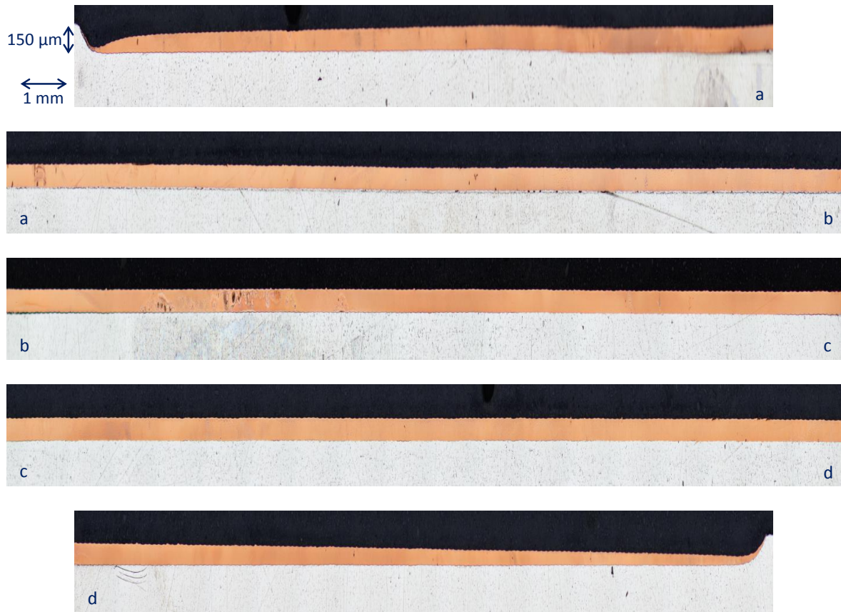
Figure 61: Longitudinal layer profile of deposited copper.
