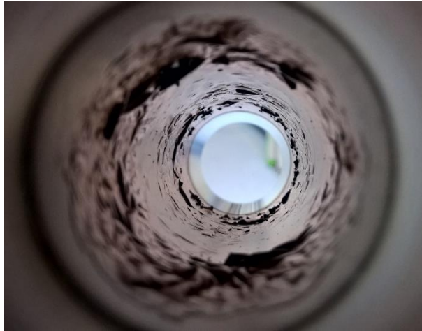
Figure 69: Copper on a zirconium layer. View inside a substrate cylinder after applying a copper layer on a previously sputtered zirconium layer.
