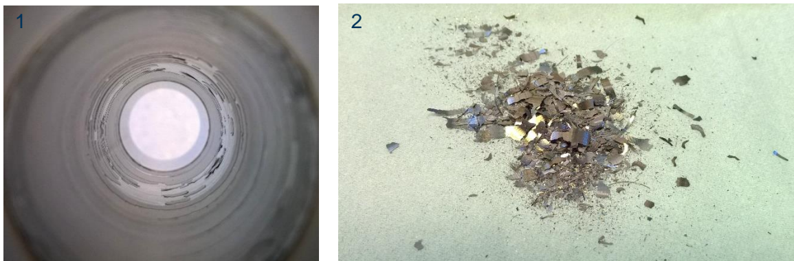
Figure 70: Flaking of zirconium layers on air. View inside a substrate cylinder coated with zirconium approximately 20 minutes after exposure to air (image 1). The coating comes off in form of small flakes (image 2) due to the oxidation of the layer.
