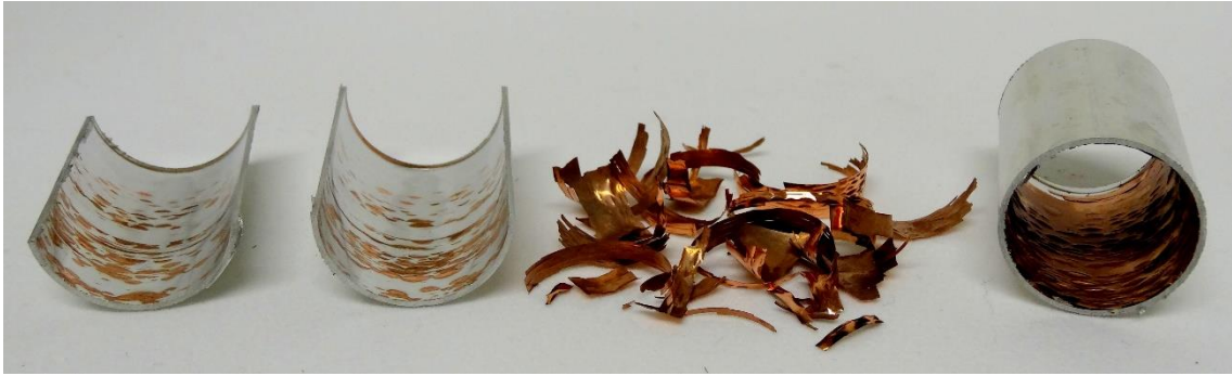
Figure 77: Copper deposited in the low energy mode. The deposited layer was very brittle and had a bad adhesion to the aluminum substrate.
