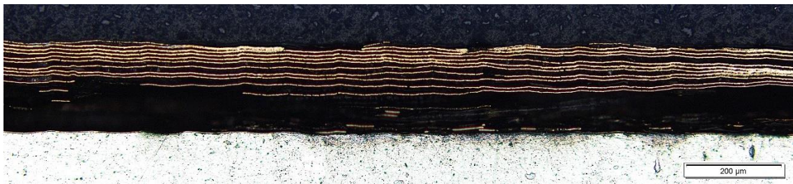
Figure 74: Deposited uranium layer. The presented layer was produced using a substrate temperature of 75°C and a sputter power of 80 W.
