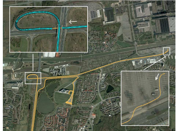
Fig. 1. Northern part of vehicle's track during test drive as determined by the proposed PPP with tight coupling of two low-cost GNSS receivers, a gyroscope and an accelerometer. The enlarged sections show the start and the passing below a bridge. Each blue point refers to a GPS-based state update.
