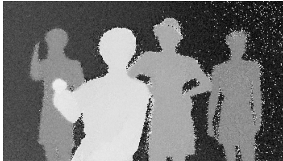
Figure 6.1: Example of a photonic mixer device TOF depth map in grayscale representation (white=0m; black=7.5m; linear in between). Crucial salt-and-pepper Noise is obvious in the right image area
