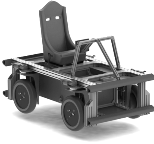
Figure 3.7: Rendering of the eCar demonstrator (adopted from [106]). On each corner, an eCorner is installed – an integrated component for steering, acceleration, and deceleration. Each eCorner can be controlled individually.
