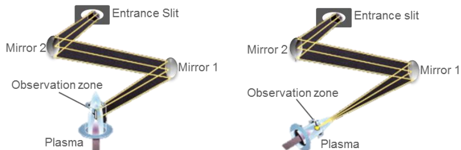
Figure 5 Radial and axial plasma viewing in ICP-OES. (adopted from Perkin Elmer brochure (Perkin)).
