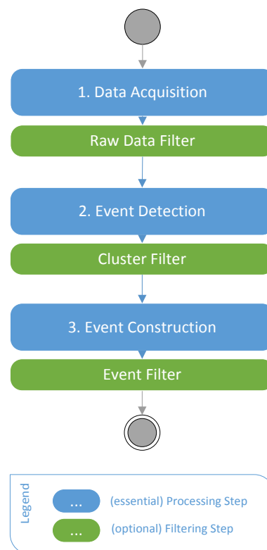
Figure 4-17: Generalized event-detection processing pipe.
