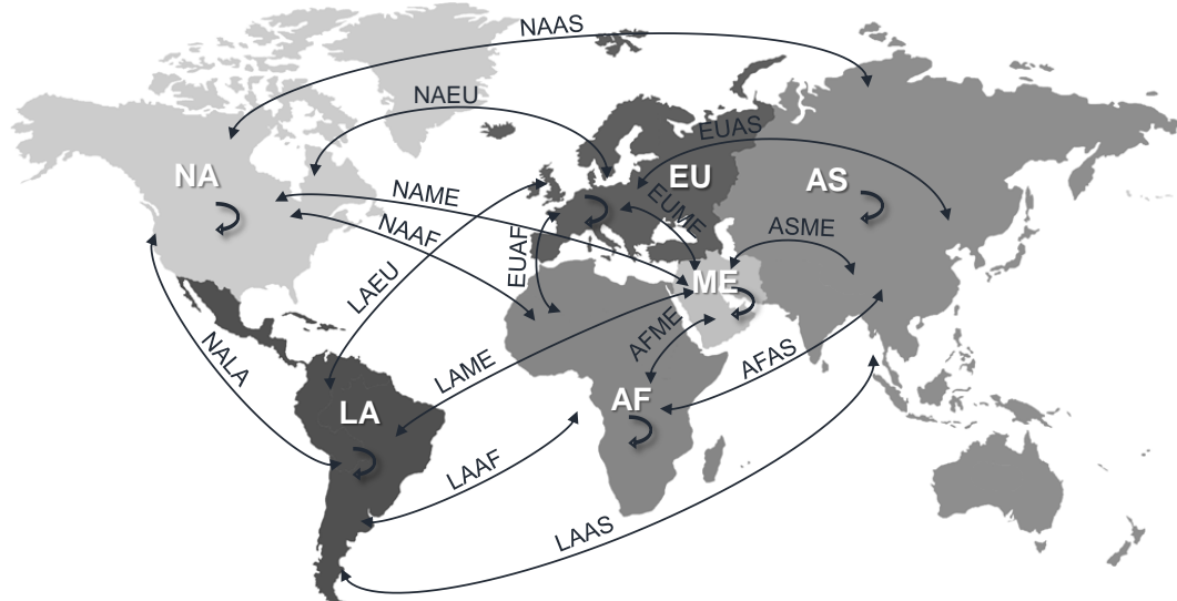
Figure 4-8 Definition of the global regions and route groups used by the FSDM Image source: world map adapted from OAG (2008)
