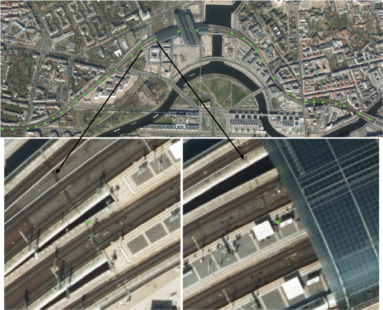
Figure 21. Upper: the midpoint of the detected railway joint cross-section marked in green, and lower: close up view of the railway joints. The background optical image has a ground spacing of 20cm.
