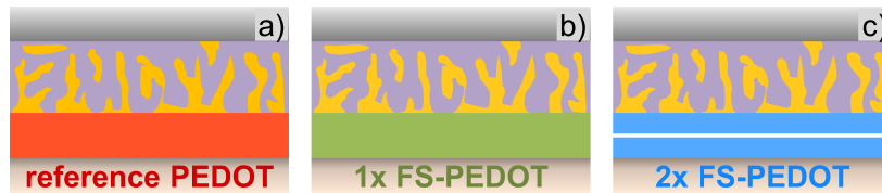
Figure 6.6: Schematic of the the investigated photovoltaic layer compositions with varying PEDOT:PSS electrodes depicted in red (a), green (b) and blue (c). a) Reference with a single pure PEDOT:PSS layer, b) solar cell with one layer of Zonyl doped PEDOT:PSS and c) solar cell with two layers of Zonyl doped PEDOT:PSS. The total PEDOT:PSS thickness is 65 nm for all PEDOT:PSS variations.
