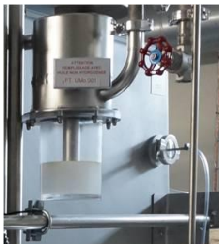
Figure 3-13 Passive pressure relief valve to protect the glovebox from excessive positive pressure.
