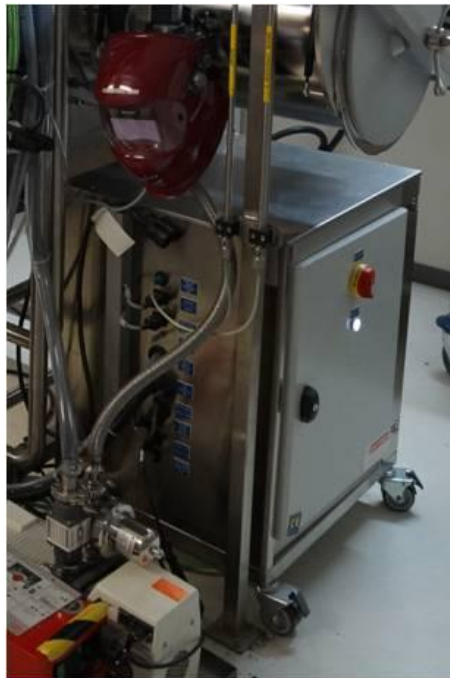
Figure 3-16 Gas purifier for glovebox atmosphere control and reprocessing.
