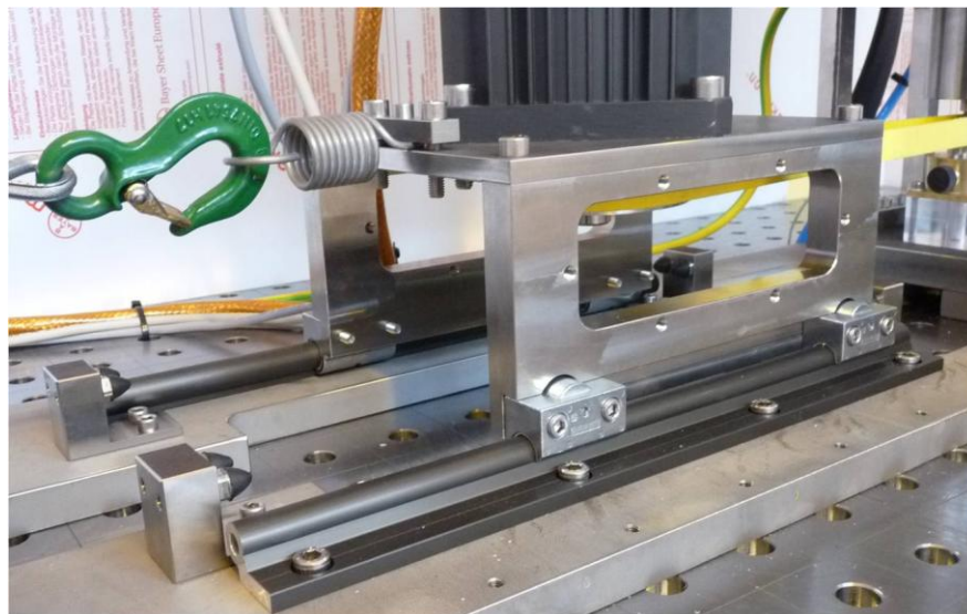
Figure 3-45 Motor carrier mounted to the hybrid bearings and linear guide rails.
