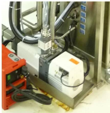
Figure 3-12 Rotary vane vacuum pump of the atomizer glovebox.
