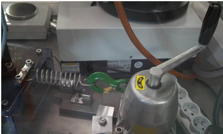
Figure 3-47 Winch with handle bar and tension spring (under load) pulling the motor carrier.
