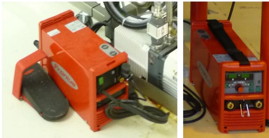
Figure 3-19 Back (left) and front view (right, showing operator interface) of the electric arc welder with foot pedal for arc ignition.
