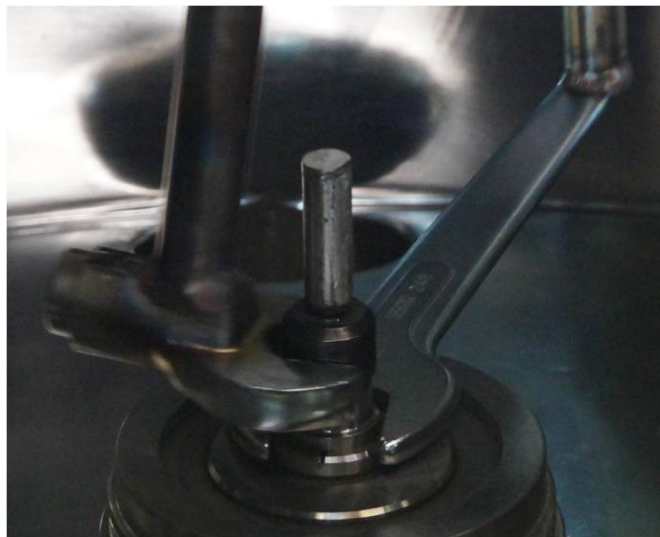
Figure 3-32 Mounting of a U8Mo rotating electrode on the collet chuck.
