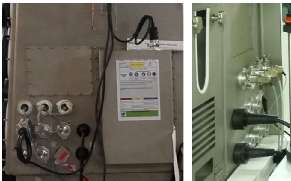
Figure 3-15 Exemplary KF40 flange fittings and feed-throughs at the atomizer glovebox backside.
