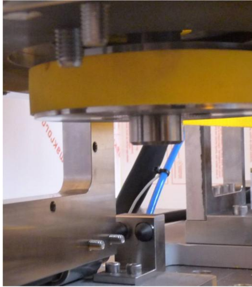
Figure 3-43 Inside view of the motor carrier showing the motor shaft, pulley, and belt (yellow).
