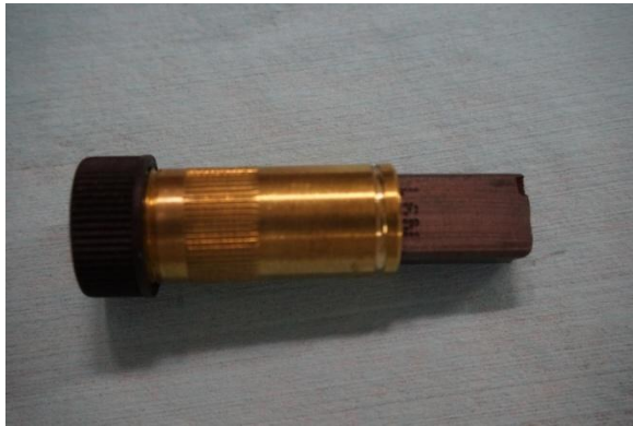
Figure 3-36 Carbon brush mounted on the brass pipe which is closed by a screwable cap at the left end.
