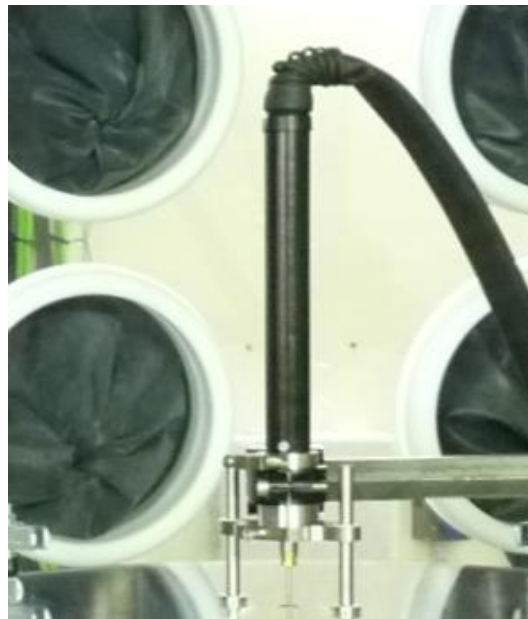
Figure 3-22 Welding torch (black bar) of the tungsten inert gas welder.
