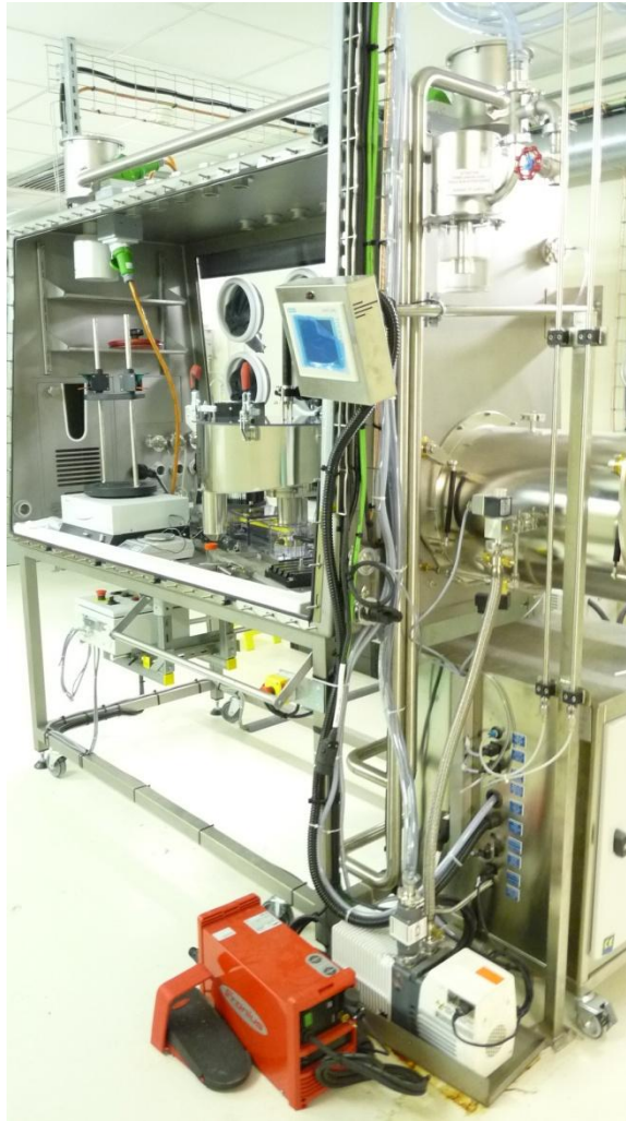
Figure 3-10 Outside view of the atomizer glovebox in the UMo laboratory before hot commissioning [Schenk et al. 2014].
