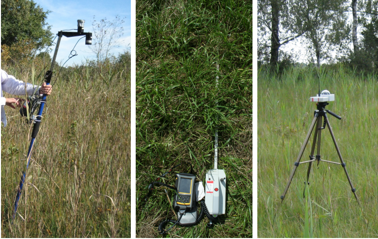
Figure 7. Left: Handheld spectroradiometer for NDVI measurements. Middle and left: Canopy analysing system for LAI measurements: The probe of the ceptometer is put underneath the vegetation (middle), whereas the beam fraction sensor (right) measures simultaneously the incoming light. The field computer (middle) calculates the LAI automatically.
