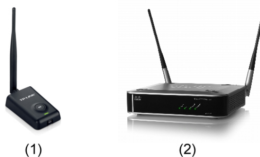
Figure 6.12: (1) is the WiFi USB adapter by TP-Link and (2) the access point by Cisco.
