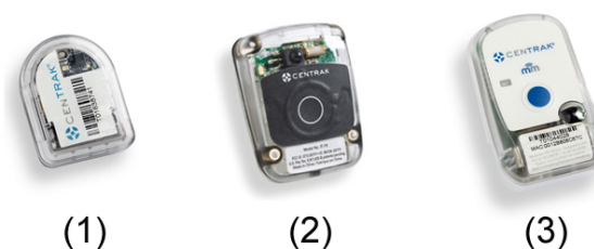
Figure 6.22: There are various tags, each with its own use case: (1) the asset tag, (2) the alert tag and (3) the patient tag.
