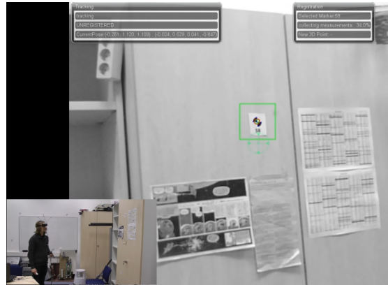
Figure 3.6: Gathering of measurements to reconstruct the 3D position of the reference points
