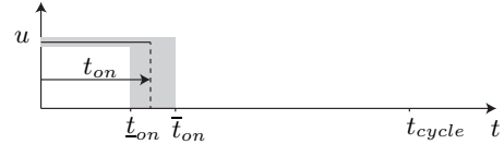
Figure 5: Range of times [\underline{t}_{on}, \bar{t}_{on}] when the charge pump is switched off. The mode both\_active is not considered in this figure.
