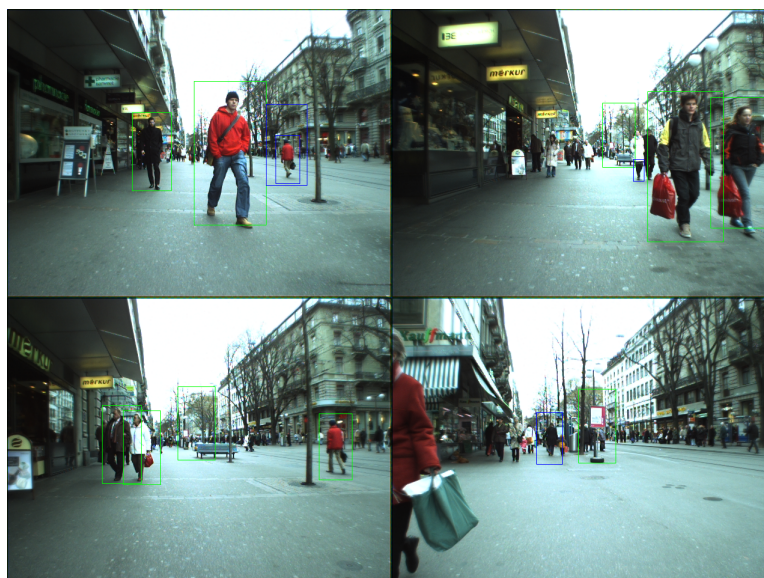
Figure 2.8: Result from Haar-Cascade and HOG algorithm
