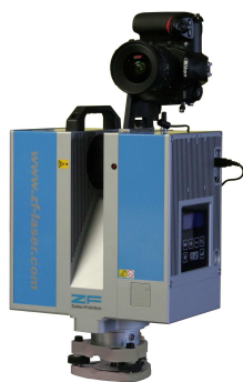
Figure 1: The Zoller+Fröhlich laser scanner Imager 5006 and a digital array camera mounted on it.
