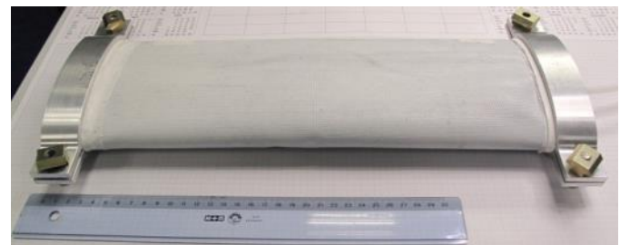
Figure 73b: Prototype before testing with elliptic, metallic end
