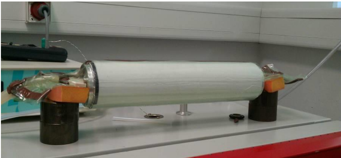
Figure 72: Prototype during manufacturing in a vacuum bag (during cool-down period)
