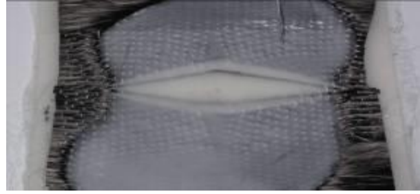
Figure 47b: Thermoplastic elastomer injected in a unidirectional 12k carbon-fiber preform at 190°C in a cast at room-temperature
