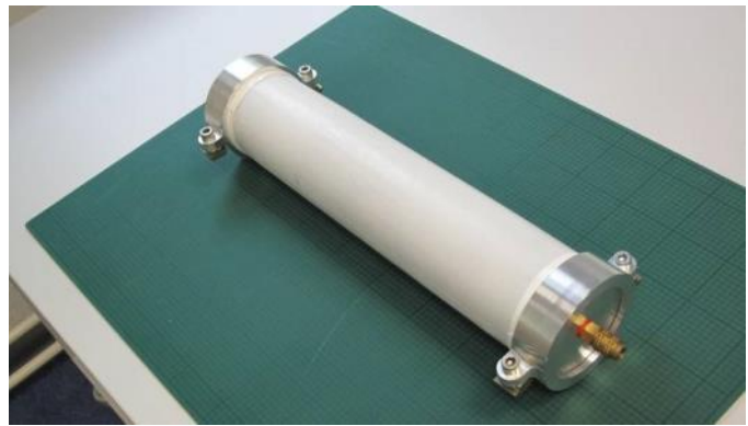
Figure 73a: Prototype before testing with round, metallic end caps
