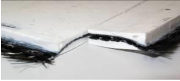
Figure 47a: TPE and carbon fibers processed in a pressure mould at 190°C at 4bar
