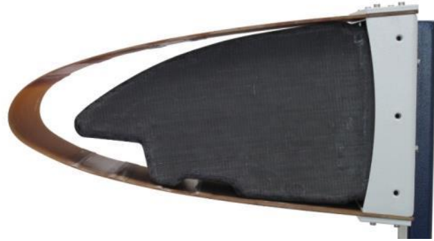
Figure 109: Completed demonstrator without actuators
