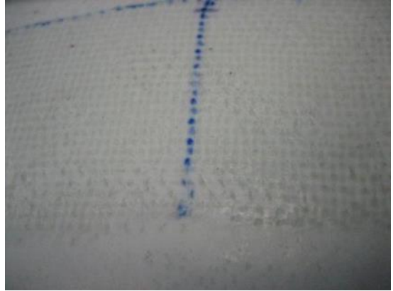
Figure 39: Woven glass-fibers in a TPE matrix
