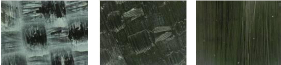
Figure 49: Carbon-fibers with a TPE matrix, after VAP (for 3h) (left and middle) and as a comparison dry fibers (right)
