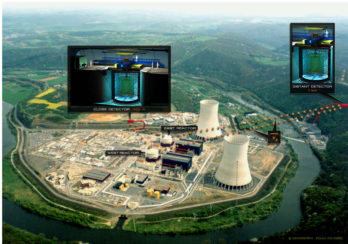
Figure 2.1: The Double Chooz experiment is located at the nuclear power plant in Chooz, a french village in the Ardennes. Each of the two reactors Chooz A and Chooz B has a thermal power of 4 250 MW. The average distance between the reactors and the neutrino detectors is approximately 400 and 1 050 meters respectively. The far detector is located in the same laboratory as the detector used in the Chooz experiment. Figure taken from [Cea10].
