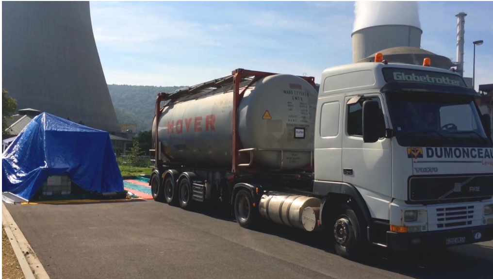
Figure 3.3: Picture of a trailer with a swap body tank used for detector liquids transportation from the LSA to the unloading area. Two swap body tanks with a nominal holding capacity of 35\text{ m}^3 each were used for the transportation of the MV and BF liquids. The picture shows the placing of the container inside a retention pit on the unloading area.
