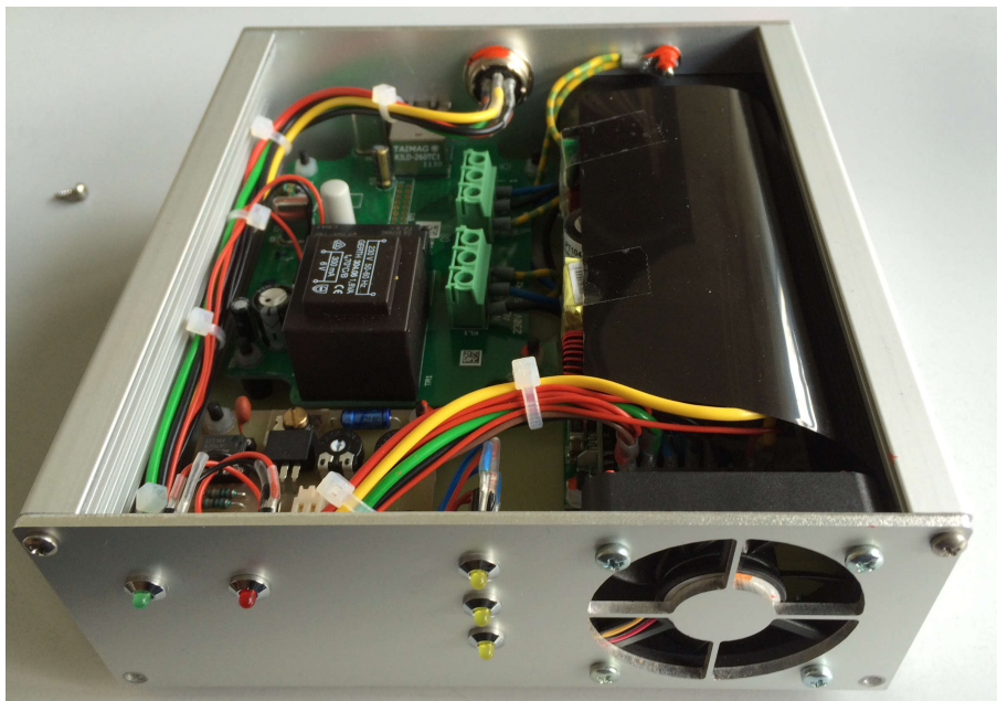
Figure 4.31: Picture of the controllable power supply which can be switched over a network connection remotely. A stabilized power supply (hidden under the black coverage) provides +5 V and +24 V, used for the LM system, and +12 V which is used to drive a temperature-dependent cooling system. The LEDs in the front plate indicate the status of the power switch (red and green) and of the different supply voltage levels (yellow).
