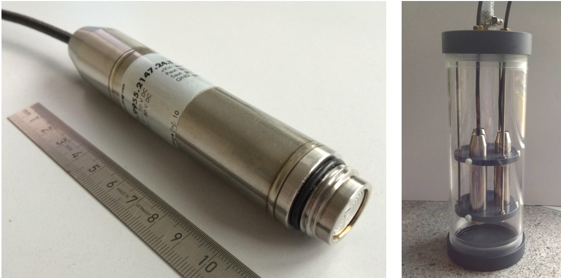
Figure 4.2: Picture of a hydrostatic pressure sensor (HPS) (left). The housing is completely made of stainless steel and the supply cable is coated with PTFE to ensure material compatibility with the liquid scintillator. It has a reader for hydrostatic pressure and temperature measurement. The sensor is able to compensate changes in liquid temperature or gas pressure above the liquid. All three sensors (MV, BF and GC) were calibrated simultaneously using an acrylic tube with a pipe filled with water at several liquid levels to ensure a proper calibration before installation in the detector (right).
