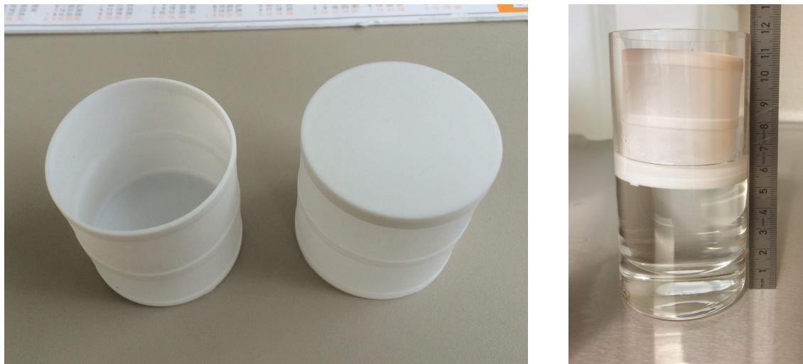
Figure 4.11: Floater as a target for the liquid level laser measurement. The turning workpiece is made out of PTFE and has very low mass due to its thin walls. It is closed with a cap to avoid flooding of the floater and has three strips on the outside to reduce friction in the guide tube (left). The upper surface for laser measurement is 40 mm above liquid level (right).
