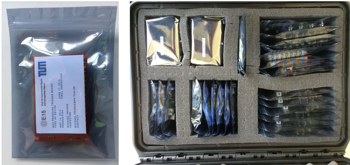
Figure 4.17: After production and testing, the electronic modules were sealed in antistatic bags together with a tag describing their function and usage in the LM system (left). All spare parts were collected together in a sealed box to protect the electronics from the high humidity in the laboratory. Spare LM computers are also included (right).
