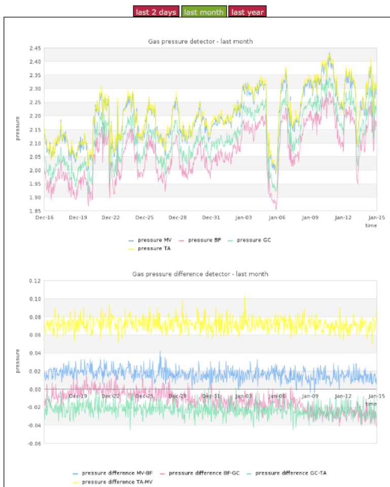
Figure 4.28: Monitoring of the near detector measurement data using a web server. The data is requested from the database, calibrated with the provided calibration data and displayed on the website. A tabular view of the latest measurement values is provided as well as a plot to show the time evolution. Three different time spans can be selected (2 days, 1 month and 1 year) as basis for the showed diagrams.
