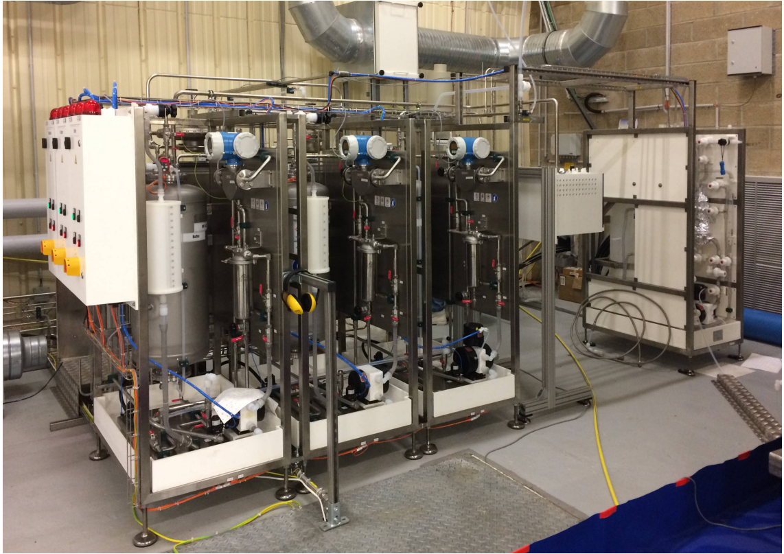
Figure 3.2: Picture of the near detector DFOS. The three modules on the left side with stainless steel components are for BF, GC and MV liquids respectively. The module on the right side with PTFE components is used for the NT liquid handling. Every module has a membrane pump, a liquid filter, intermediate tanks and a mass flow meter. The switchboard on the very left side is used to control selected valves and to start or stop the pumps included in every module. A leakage detection system will shut all valves and turn off the pumps if any liquid is detected in the white trays below each module.
